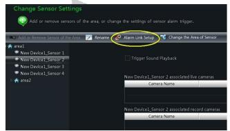
Click "Add Associated Record Camera" to choose associated record cameras. When the sensor alarm is triggered, the selected cameras will be recorded automatically.
