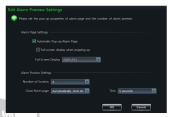
drop-down menu. The alarm image will display on the designated monitor when alarm is triggered. Set the number of screens. You can choose to close the alarm page automatically or manually. You can set the time if auto mode is selected.
