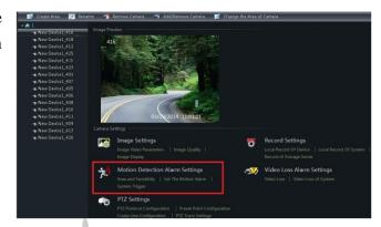
Select a camera and then click *Set Motion Alarm* under Motion Detection Alarm Settings to go to the interface as shown on the right. Enable Alarm of device and set the relevant trigger.
