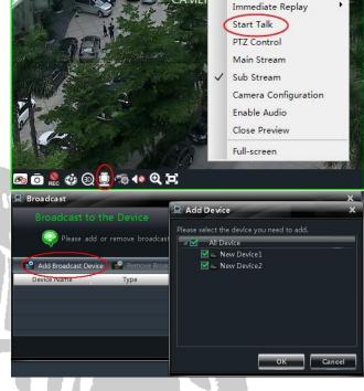
Click "Add Broadcast Device" button to pop up a window and then check the devices you want to broadcast. Click "OK" button to save the setting. Click "Start Broadcasting" to start broadcasting.
