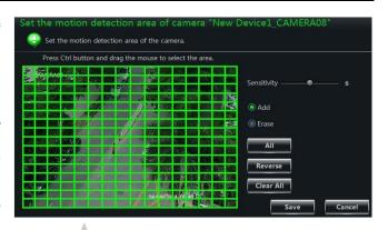
Click *Set The Motion Alarm* to go to the interface as shown on the right. You can set the motion alarm and linkage configuration.
