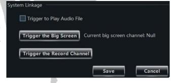
Click "Trigger the Big Screen" button to select channel. If the motion alarm of the selected channel is triggered, a big picture will pop up on the screen.
