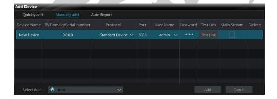
There are three modes available for you to add device ("IP Address", "Domain name" and "Serial number"). You can add the device which supports NAT function through "Serial number".
