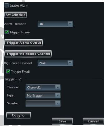
Click *System Trigger* under Motion Detection Alarm Settings to go to the interface as shown on the right.
